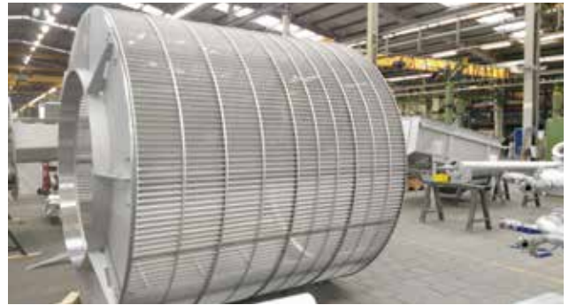
ROTAMAT® STAR screen basket, 2600 mm diameter, 1 mm perforation, acid-treated in a pickling bath and passivated.
